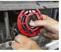
Due to the size of the new super-tone horns, check the optimal assembly position. The housing body must have sufficient leeway for swinging into all directions and should be in contact with the adjacent body parts.
