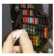
Remove the fuse for the "Horn" circuit from the fuse box in order to cut the power supply of the acoustic signaling units for the duration of the electric
